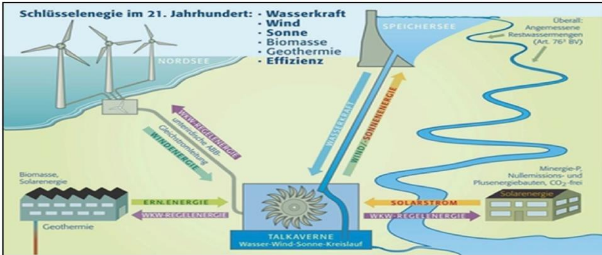
Fig. 7: Pumped-storage power plants (PPT) pump solar power surpluses during the day and high wind power surpluses in winter into existing or renovated storage lakes. At night, when there is no wind and on days with little sunshine, the PPT can generate CO 2 -free electricity in the GW range for Central Europe (cf. PEB building study 2019, pp. 67-69).
